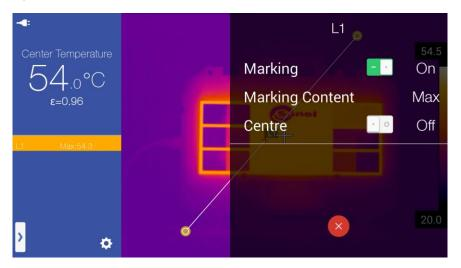
The 'Marking' option turns on/off the temperature points displayed on the line. The 'Marking Content' option allows to select the displayed temperature value for the line: minimum, maximum or average. The 'Center' option moves the line to the center of the screen.
