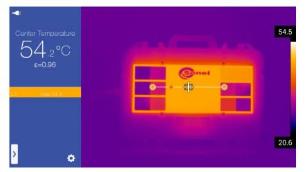
The shape and the position of the line can be modified (rotate, lengthen, shorten). This can be done by changind the position of its endpoints. This can be done by pressing and
