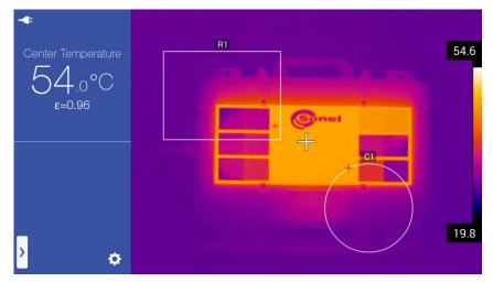
The shape and the position of the object can be modified (rotate, lengthen, shorten). This can be done by changing the position of its defining points. Press and hold the selected
