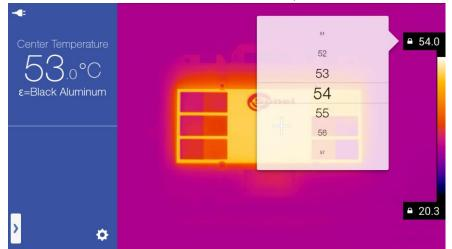
After selecting desired value, close the temperature selection window by clicking anywhere outside its outline. Moreover moving the joystick [18] up or down sets both temperature range values. Clicking the joystick activates the focus adjustment (chapter 3.3). Press A/M (22) button to switch into automatic temperature selection mode.
