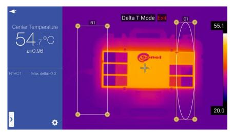
The calculated temperature difference is isplayed on the left side of the screen, in the additional information field [G]. If the difference is for the maximum temperatures, the result is described as Max Delta, for the minimum temperatures as Min Delta and for medium temperatures an Average Delta. The calculation method is always the same, and the description alone indicates only the type of the temperatures for which the difference was calculated.
