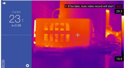
After the countdown is finished, the camera will start recording video, with the entire procedure and the screen layout during the process being the same as in the manual mode. After the video recording, with predefined time, is finished, the camera will automatically end the recording procedure, save the video into the memory, and will resume its operation in real time mode.
