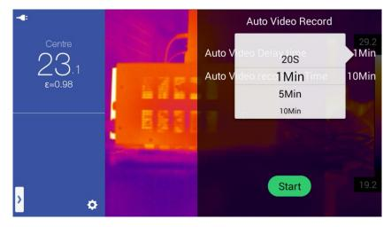
After setting the parameters, start the video recording by pressing on-screen START button. In the upper right corner of the screen the camera will display notification on its readiness to commence video capturing, along with the information on the time that left before
