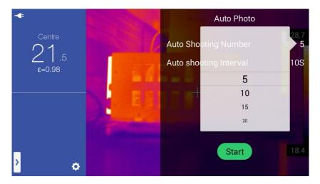
After setting the parameters, start the automatic capture of images by pressing on-screen START button. The camera will then take predefined number of images and will store them into memory, resuming its operation in real time mode afterwards.
