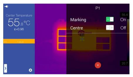
The 'Marking' option turns on/off a description of the spot marker. The 'Center' option moves the spot to the center of the screen.
