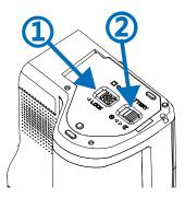
Push the battery lock lever above the battery and the battery will partially slide out of the compartment, allowing to remove it.
