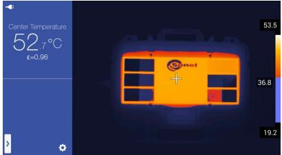
The boundary temperature change is possible by pressing and holding down the boundary temperature tag on the temperature bar. A speech bubble, with the temperature value, will appear on screen. Select the desired temperature by sliding the marker up (to increase the temperature) or down (to decrease the temperature).
