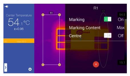
The 'Marking' option turns on/off the temperature points displayed on the line. The 'Marking Content' option allows to select the displayed temperature value for the object: minimum, maximum or average. The 'Center' option moves the object to the center of the screen.
