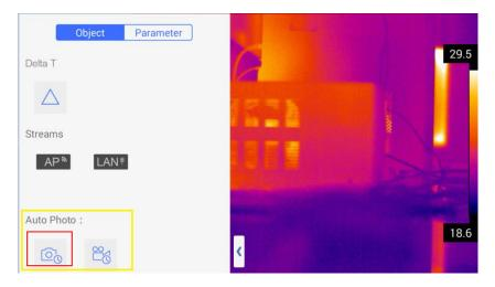
Press Auto Photo icon  $\bigcirc$  to open up a menu that allows to set a number of images to be taken and the time interval between them. To change these parameters click the value of each parameter individually.
