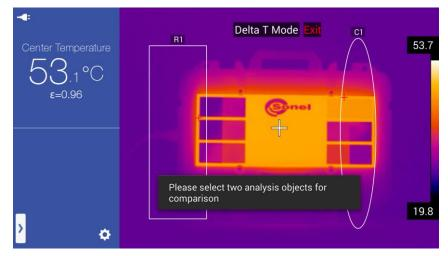
Select the two objects, for which the temperature difference will be calculated. This is done by clicking any area of the first object and then any area of the second one.
